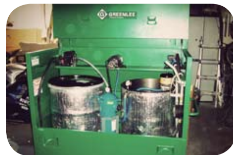
3. Filter vegetable oil and pump SVO into vehicle.
